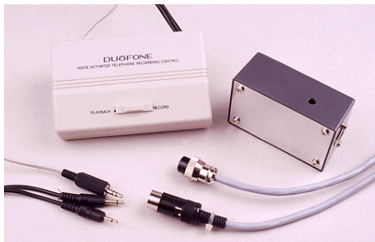
Figure 2—The VOX unit and the interface box. The VOX unit's PHONE LINE cable connector is rigged to terminate in a three-circuit phone jack. The two miniplugs are from the VOX unit RECORDER output. The DIN plug at the right of the relay box routes mike audio, ground and two PTT-line wires to the rig's mike connector.
